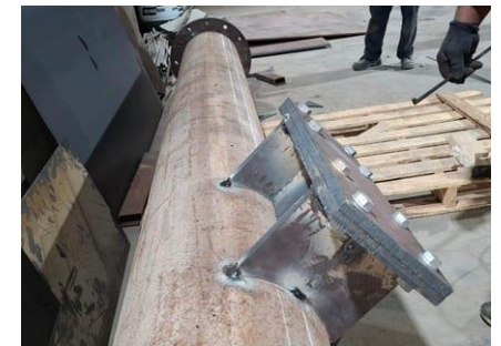
Column base connection. Case study D, page 12.
