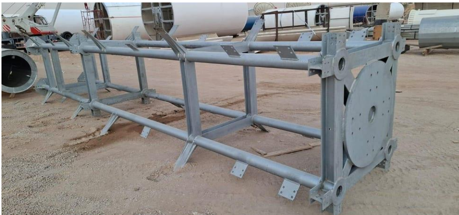
Galvanized tower-top frame with mounting plate and bracing.
