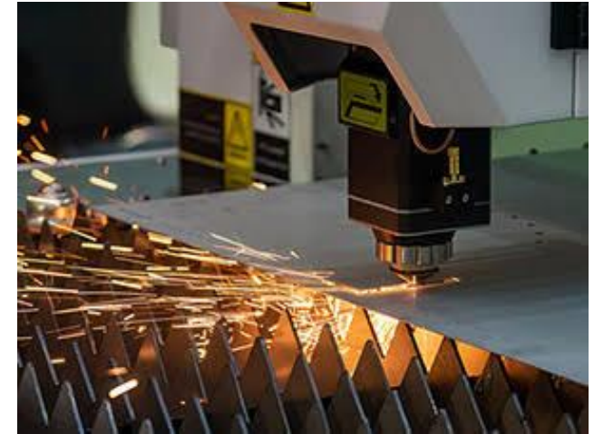
Patterned panels cut on the flat laser bed. Case study A.
