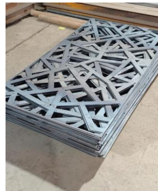
Finished panels stacked for handling. The pattern is cut through the plate.
