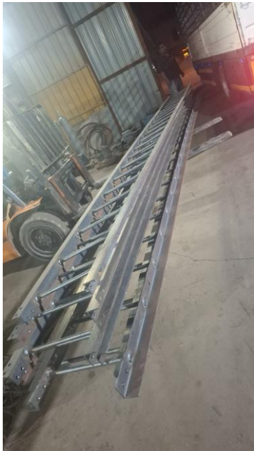
Drilled connection holes along the stringer flanges.
